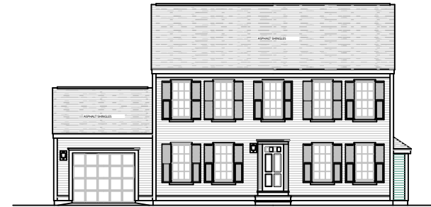
FRONT ELEVATION SCALE 1/4" = 1'-0"
